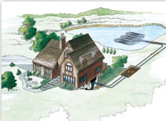
An example of a pond loop installation
