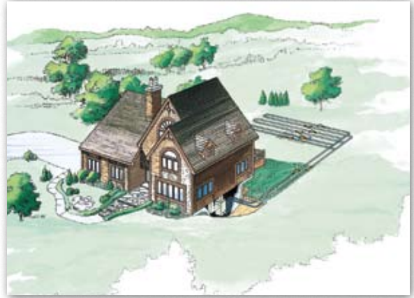
An example of a horizontal loop installation
