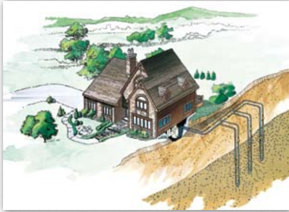
An example of a vertical loop installation
